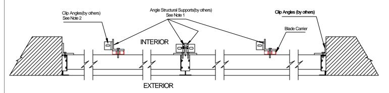
WHEN INSTALLING FROM INTERIOR SIDE OF OPENING , THE END PANELS ARE FABRICATED WITH VISIBLE JAMB SECTIONS ON BOTH ENDS AND A BLADE CARRIERS AT THE MAXIMUM FO 5 FT CENTERS.
